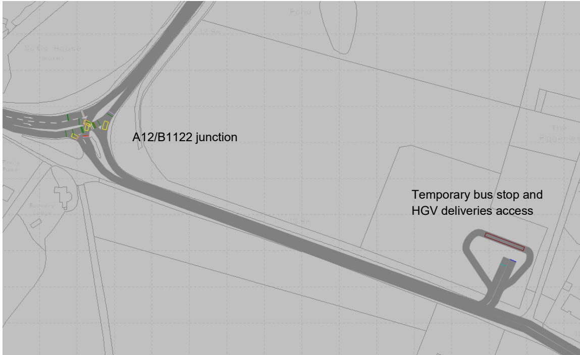
Figure 24 – Temporary bus stop and HGV delivery access at Yoxford junction
